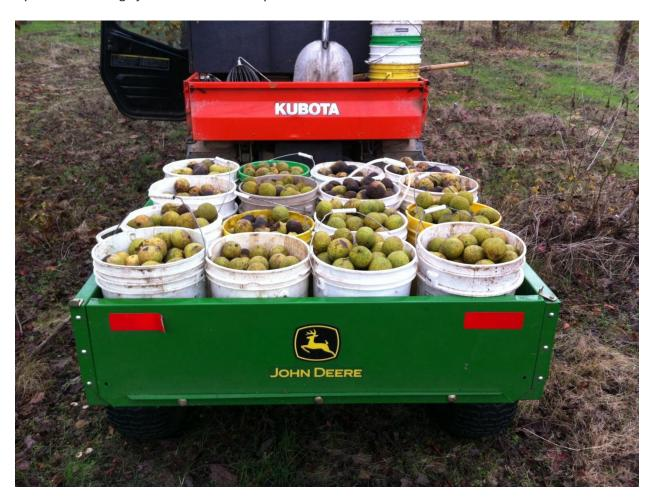
2. When we get 16 buckets full, a cart hauls them to our homemade huller. The huller is direct drive from a tractor PTO. It doesn't take much power. We run the engine speed at 1500 rpm for wild nuts and 1000 for thin shelled cultivars - any faster will crack them. We speed up until we start racking nuts.
